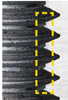
Detailed view with burrs along threads
